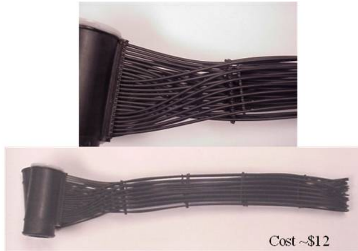
Figure 44. Prototype low-cost polymer HX. Tubes are 1/8 in. (3 mm) diameter. Tube production, tube weaving, and tube-to-header welding are automated processes, contributing to a low-cost projection.
