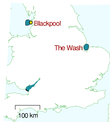
Figure 14.9. Two tidal lagoons, each with an area of 400 \text{ km}^2 , one off Blackpool, and one in the Wash. The Severn estuary is also highlighted for comparison.
