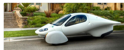
Figure 20.40. The Aptera. 6 kWh per 100 km . Photo from www.aptera.com .
