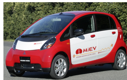
Figure 20.38. The i MiEV from Mitsubishi Motors Corporation. It has a 47 kW motor, weighs 1080 kg, and has a top speed of 130 km/h.
