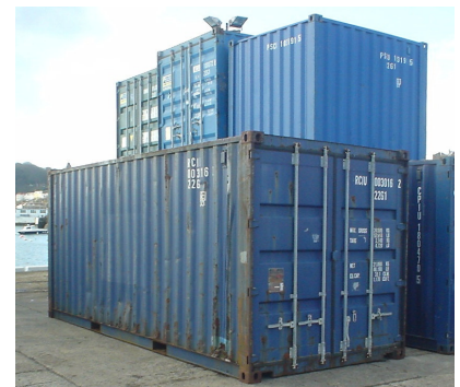
Figure I.4. A twenty-foot container (1 TEU).
