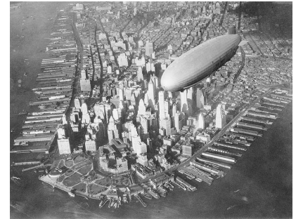
Figure C.14. The 239 m-long USS Akron (ZRS-4) flying over Manhattan. It weighed 100 t and could carry 83 t. Its engines had a total power of 3.4 MW, and it could transport 89 personnel and a stack of weapons at 93 km/h. It was also used as an aircraft carrier.
