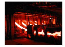
Figure H.1. Continuous casting of steel strands at Korea Iron and Steel Company.
