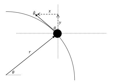
We can use the same logic we used before to figure out x and y, using sine and cosine. Notice however that the x is now opposite and the y is now adjacent.
