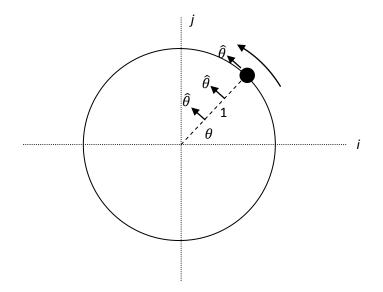
The first thing to determine is which way the  $\hat{\theta}$  is pointing. The  $\hat{\theta}$  is the angle opening up as the object revolves around the circle. It always points perpendicular to  $\hat{r}$  as is shown above.
