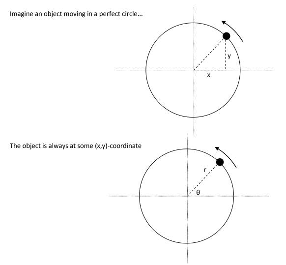
Or we can say the object is at a (r,  $\theta$ ) coordinate where r is the radial distance from the center of the circle and  $\theta$  is the angle shown above.
