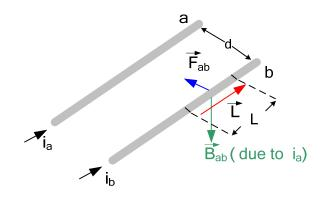
The magnetic filed due to i<sub>a</sub>:
