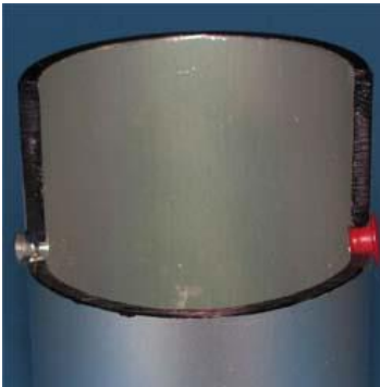
Eyelets do not protect the line from the inside edge.
