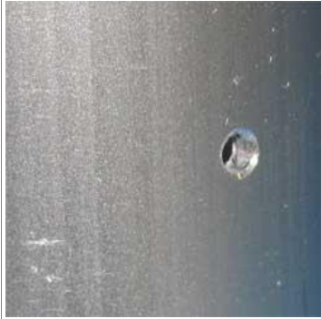
Chamfer outside hole using an oversized drill bit.
