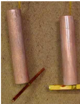
First coat of toilet bowl cleaner containing hydrochloric acid has been applied. Dried in about two days
