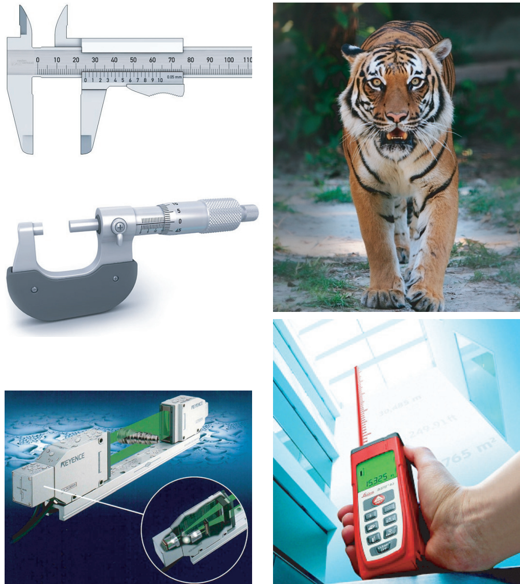
FIGURE 23 Three mechanical (a vernier caliper, a micrometer screw, a moustache) and three optical (the eyes, a laser meter, a light curtain) length and distance measurement devices (© www.medien-werkstatt.de , Naples zoo, Leica Geosystems and Keyence)
