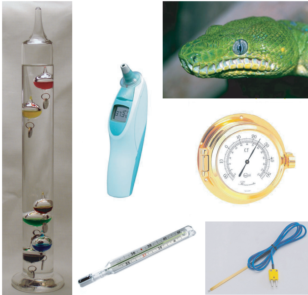
FIGURE 202 Thermometers: a Galilean thermometer (left), the row of infrared sensors in the jaw of the emerald tree boa Corallus caninus , an infrared thermometer to measure body temperature in the ear, a nautical thermometer using a bimetal, a mercury thermometer, and a thermocouple that is attached to a voltmeter for read-out (© Wikimedia, Ron Marcus, Braun GmbH, Universum, Wikimedia, Thermodevices)
