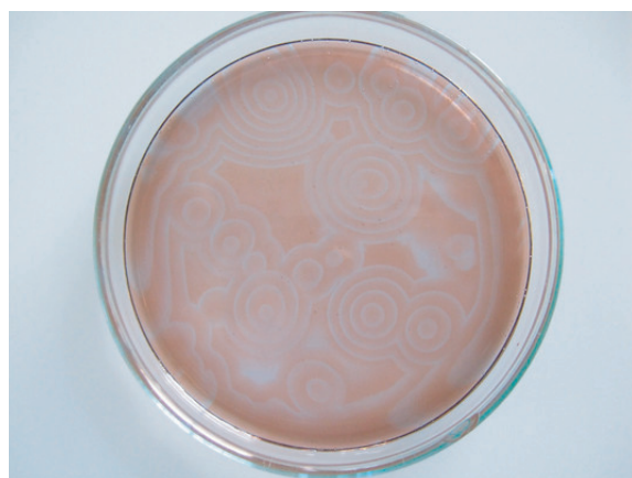
FIGURE 223 The Belousov-Zhabotinski reaction: the liquid periodically changes colour, both in space and time. (© Yamaguchi University)
