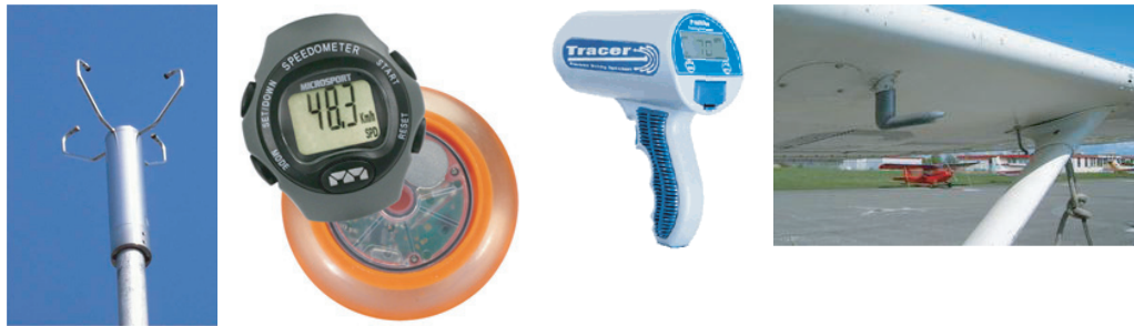
FIGURE 16 Some speed measurement devices: an anemometer, a tachymeter for inline skates, a sport radar gun and a Pitot-Prandtl tube in an aeroplane (© Fachhochschule Koblenz, Silva, Tracer, Wikimedia)
