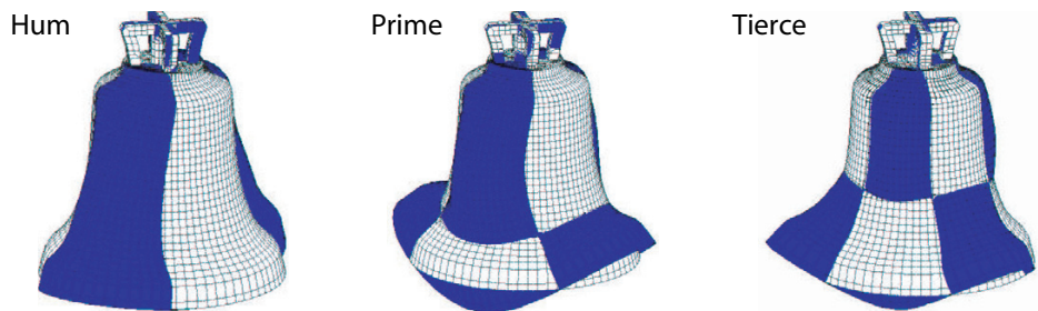
FIGURE 160 The measured fundamental vibration patterns of a bell. Bells – like every other source of oscillations, be it an atom, a molecule, a music instrument or the human voice – show that all oscillations in nature are due to waves. (© H. Spiess, al).
