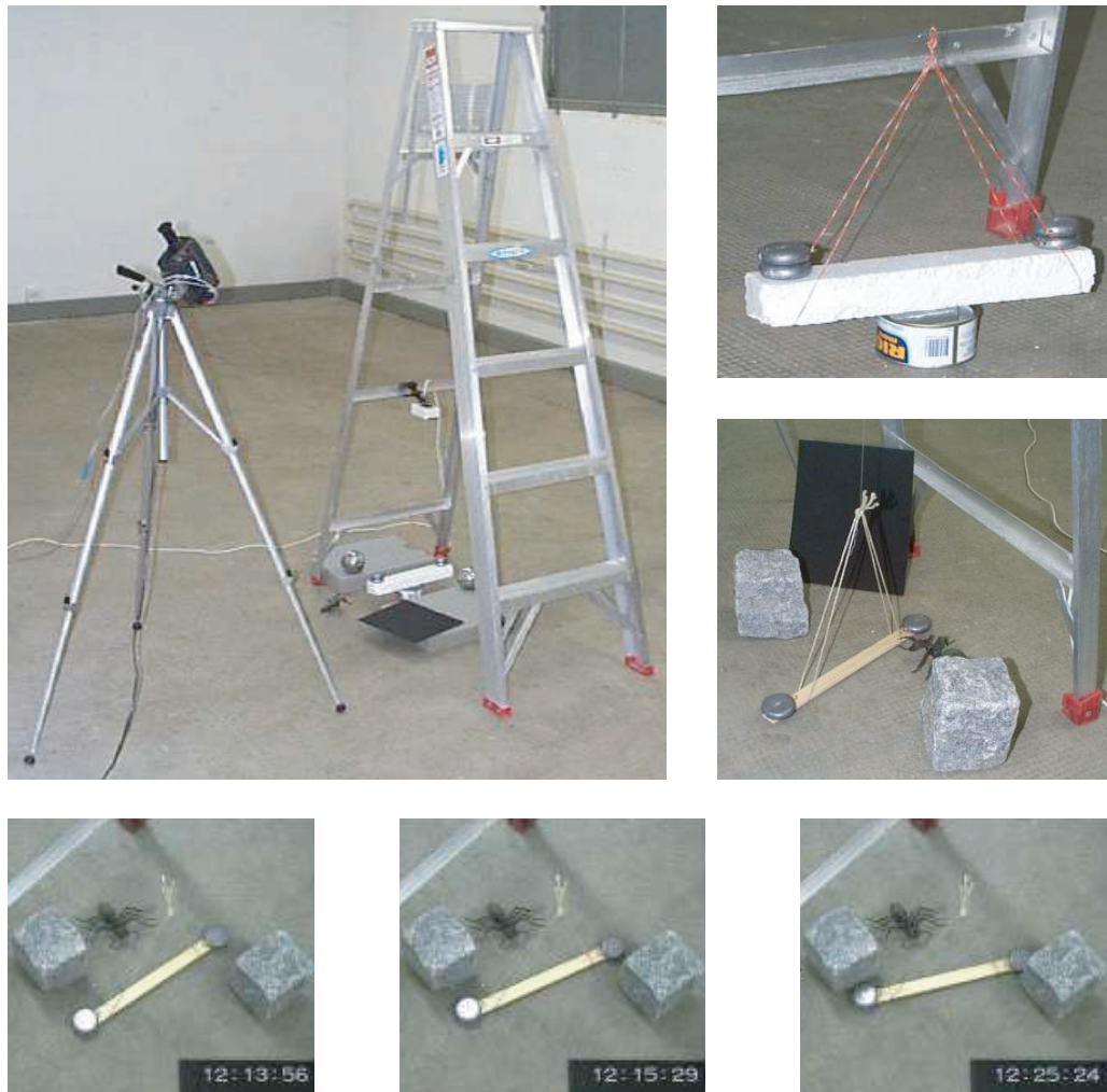
FIGURE 108 An experiment that allows weighing the Earth and proving that gravity also works sideways and curves space. Top left and right: a torsion balance made of foam and lead, with petanque masses as fixed masses; centre right: a torsion balance made of wood and lead, with stones as fixed masses; bottom: a time sequence showing how the stones do attract the lead (© John Walker).
