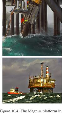
Figure 10.4. The Magnus platform in the northern UK sector of the North Sea contains 71 000 tons of steel. In the year 2000 this platform delivered 3.8 million tons of oil and gas – a power of 5 GW. The platform cost £1.1 billion. Photos by Terry Cavner.
