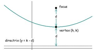
5) The geometry of a parabola is special in that it focuses parallel beams of light or radiation toward a single point. The form of this parabola is given by
